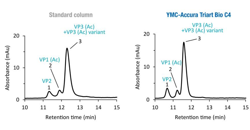
Both, the YMC-Accura Triart Bio C4 and the standard YMC-Triart Bio C4 column enable the separation of the AAV capsid proteins VP1 and VP2. The bioinert YMC-Accura Triart Bio C4 additionally prevents
