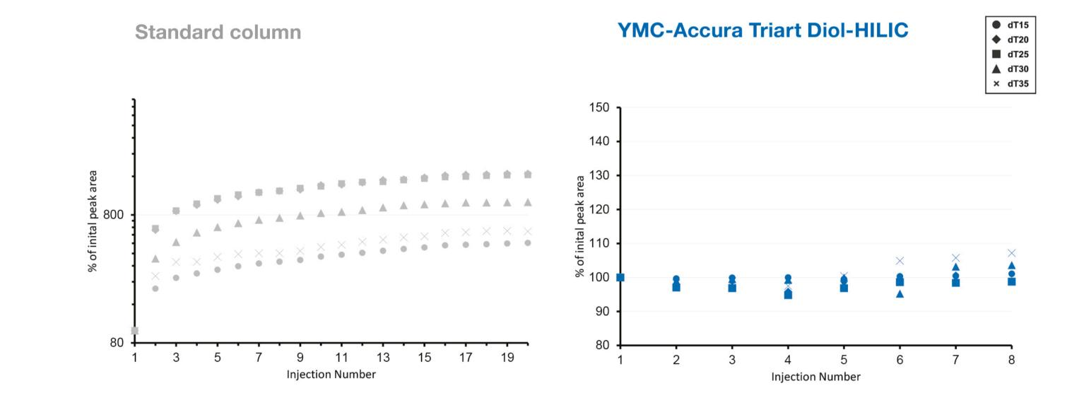
The bioinert YMC-Accura Triart Diol-HILIC needs only 8 injections for conditioning, assessed by the difference between the initial and 8th peak area being less than 10 % [1]. In contrast, with the stainless steel column, 20 injections are required until full conditioning is achieved [2].
