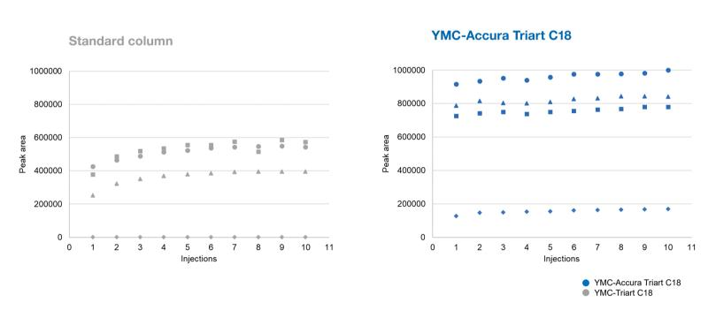
Analysis of phosphorylated peptides with the bioinert YMC-Accura Triart C18 column gives very stable peak areas. About 6-9 % deviation is seen for T18p, T19p and T43p within the first 10 injections. In comparison, the standard stainless steel column shows deviations of up to 56 %.
