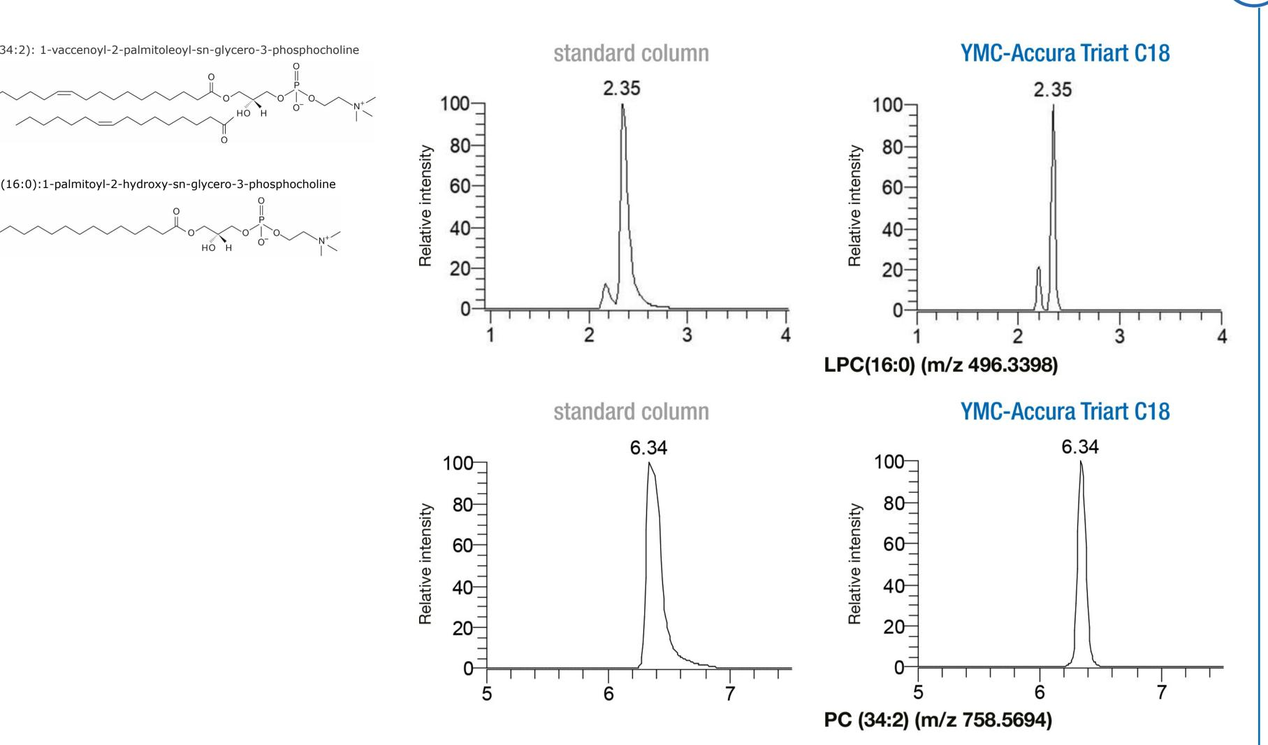
YMC-Accura Triart C18 (1.9 µm, 12 nm) 100 x 2.1 mm ID
