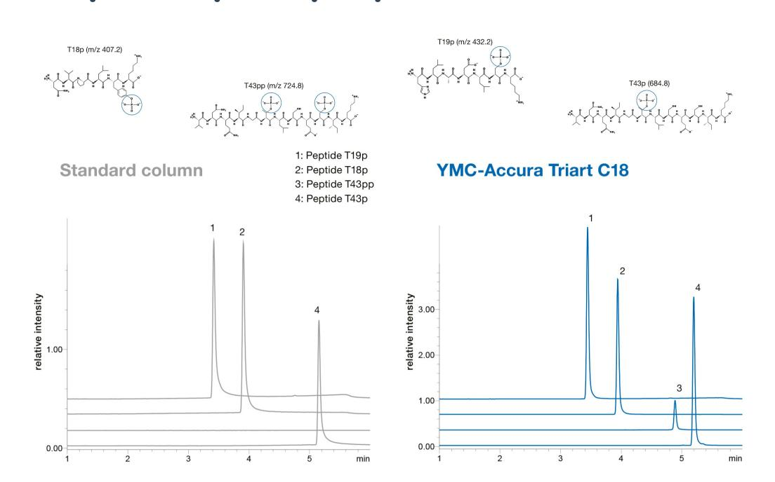
The use of the bioinert YMC-Accura Triart C18 column led to higher intensities and peak areas for all peaks. Due to the high recovery rates of YMC-Accura Triart C18 the challenging phosphopeptide T43 pp, which contains two phosphate residues, can be detected. This is not achieved using the standard stainless steel column.
