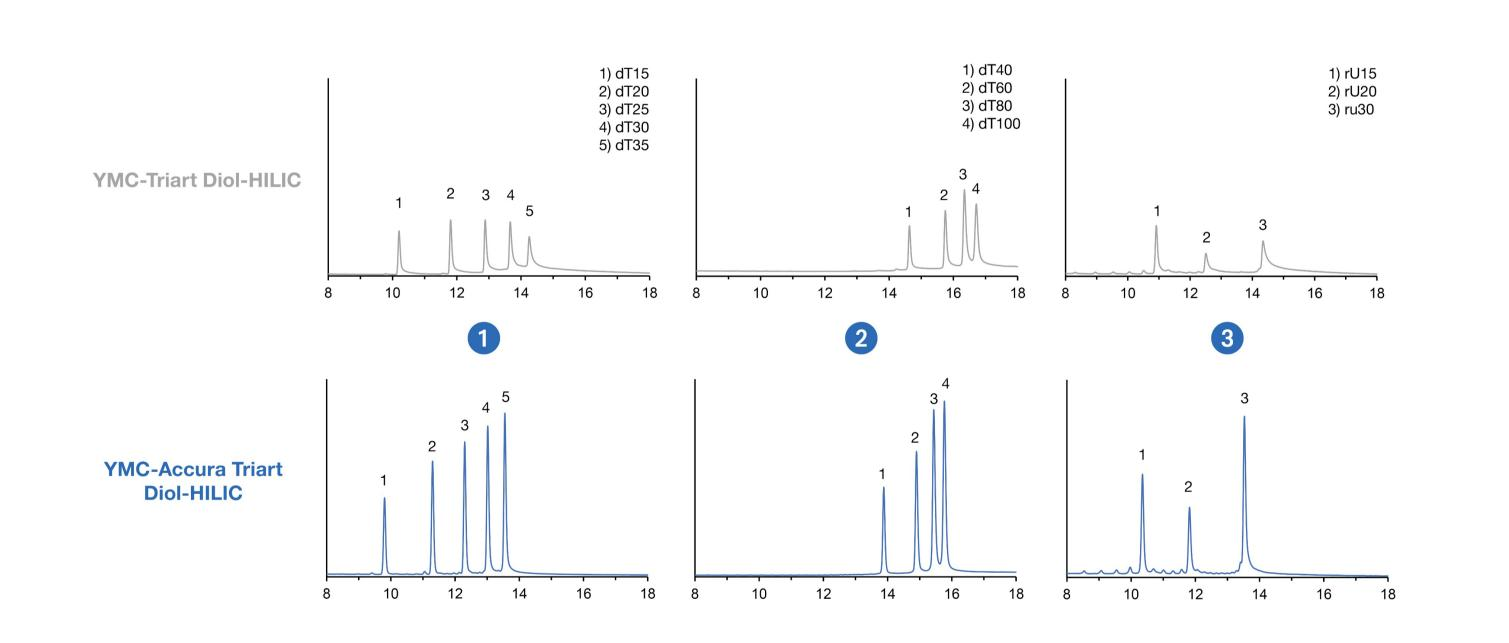
Use of the bioinert YMC-Accura Triart Diol-HILIC column results in higher sensitivities, peak areas and less tailing for all sizes and types of nucleotides tested [1]. Non-specific adsorption did not vary according to nucleotide length, even though the adsorption is usually higher for longer oligonucleotides in IP-RP. On the contrary, the relative peak areas varied strongly for the stainless steel column, which indicates that non-specific absorption is still significant [2].
