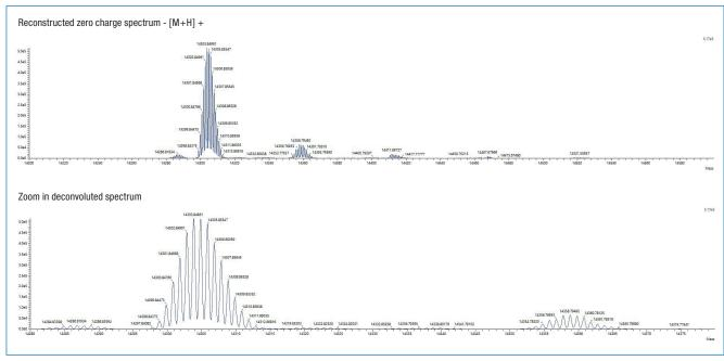
Figure 2: Deconvoluted spectrum of lysozyme (2) at the retention time of 4.85 min.
