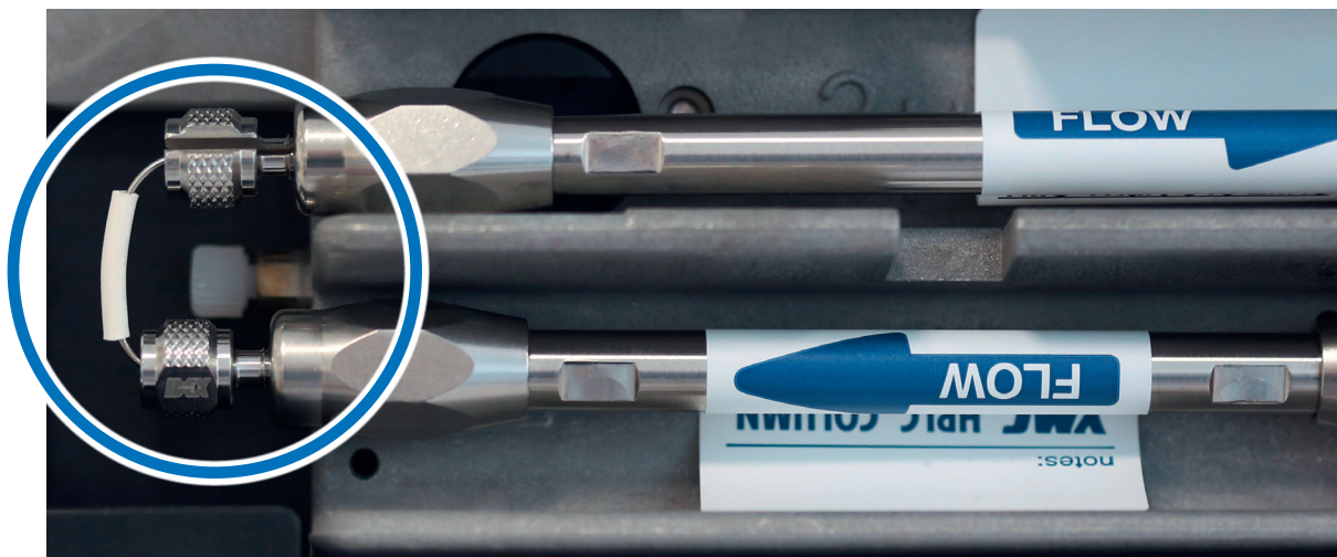
Coupling of two YMC-Triart UHPLC columns using the dead volume free MarvelIX™ connector.
