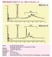
Two different lots of commercially available MAb, purified by DEAE chromatography, are separated on 100 mm length-column packed with non-porous polymer beads. The MAb is resolved into several peaks and the lot-to-lot variability is observed. The 100 mm-length column of YMC-BioPro QA-F and SP-F has high efficiency and it is ideal for characterization or QC assessment of closely related proteins.
