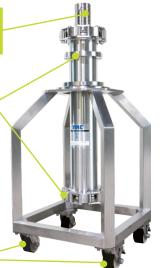
The YMC-Actus SP uses a cylinder to pack the packing material by physical compression. The piston is fixed in place after compression. After packing, the packed bed is kept compressed by a spring in the piston. Therefore, it provides higher pressure resistance and durability.
