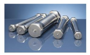
YMC-Actus preparative columns were developed by applying this same technology. The column bed is compressed when attaching the inlet end assembly of the YMC-Actus hardware. This provides increased bed density (10% higher than that of conventional columns) and bed uniformity. Packed with YMC resins, Actus columns have been shown to maintain high stability under high flow rates and steep gradient conditions.
